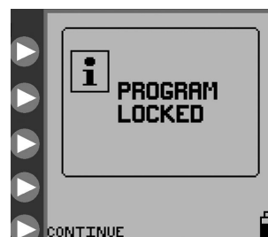
Figure 16. Program Locked screen, which indicates the pump is in LOCK SETTINGS mode.
